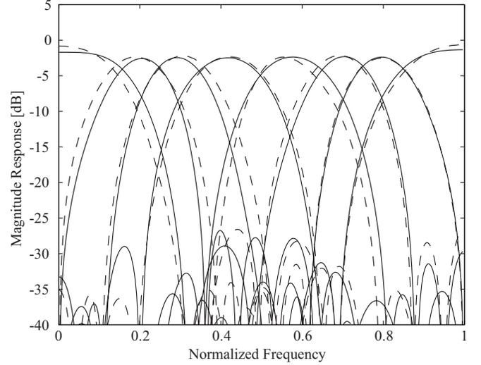
Fig. 3. Comparison between Design examples for the analysis banks of the Type 1.3 OLPPRFB with  $K_0 = K_1 = 1$  and  $N = 3$  (solid line) and the pre- and postprocessing system [6] with  $K_1 = 2$  (dashed line), both have  $P = 8$ ,  $M = 6$  and  $L = 36$ .
