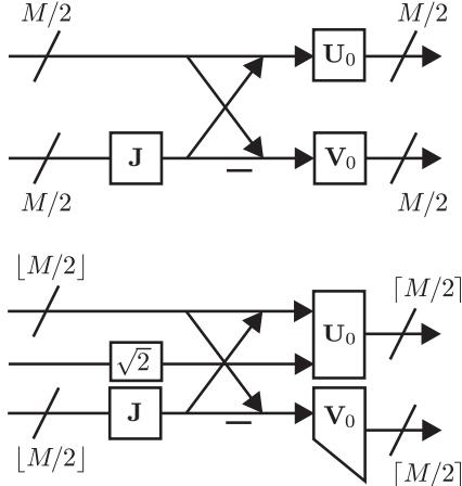
Fig. 1.  $\tilde{\mathbf{Q}}_0$  for Type 1.3 OLPPRFBs: (Top)  $\tilde{\mathbf{Q}}_0$  for even  $M$ . (Bottom)  $\tilde{\mathbf{Q}}_0$  for odd  $M$ .
