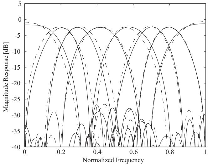
Fig. 3. Comparison between Design examples for the analysis banks of the Type 1.3 OLPPRFB with  $K_0 = K_1 = 1$  and  $N = 3$  (solid line) and the pre- and postprocessing system [6] with  $K_1 = 2$  (dashed line), both have  $P = 8$ ,  $M = 6$  and  $L = 36$ .
