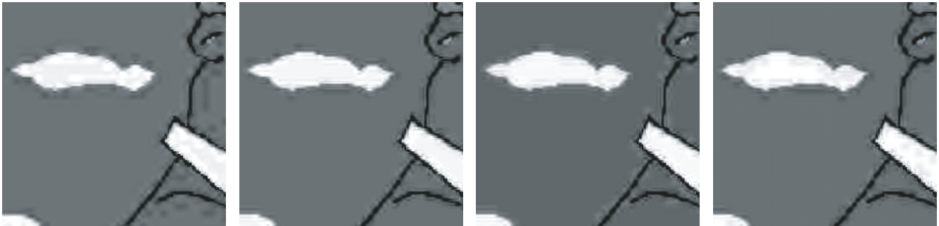
Fig. 3. Comparison of reconstructed images (1:32, portions of Yogi ). From left to right: 9/7 DWT, 8 \times 16 BOLPFB, FOLPFB, UFLPFB.
