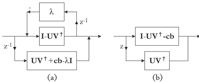
Figure 4: The structure of Order-1 IIR-FIR hybrid building blocks:(a) analysis filter (b) synthesis filter.
